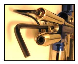
Note that you will not remove the banjo bolt from the front block. The front block will move away from the marker as you remove the banjo bolt and allow you to remove it.
